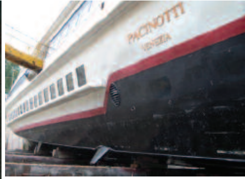
Condition of a fast vessel coated with Intersleek 425, 5 years later.
